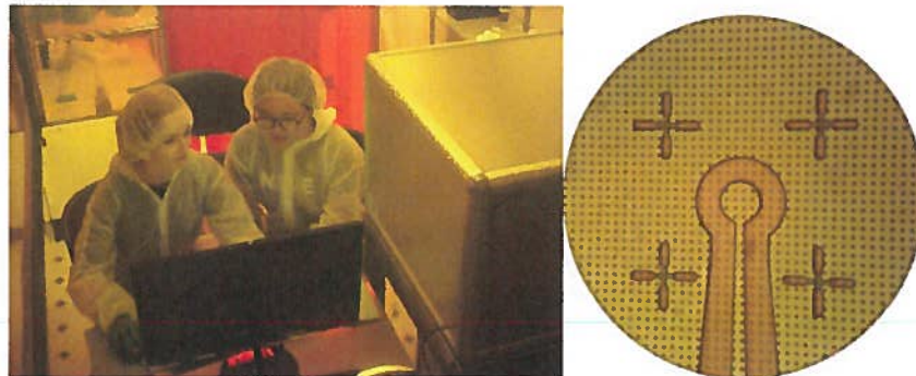
Fig. 1: Fiona McCluskey (left) and Tori Dang (right), undergraduate students from Bryn Mawr College who worked at CSU for Kristen Buchanan's group last summer, are patterning copper hoops for research on the effects of Dzyaloshinskii Moriya interactions (DMIs) on spin dynamics and on skyrmion formation. The samples will be characterized using micro-focus Brillouin light scattering. The image on the right shows a patterned hoop in S1813 on top of magnetic structures made by Tori and Fiona using the lithography system. The hoop inner diameter is 20 \mu\text{m} . The smaller circles are patterned multilayered magnetic structures that will be used to study the effects of DMI on spin dynamics.
