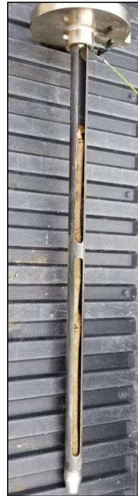
Figure 3.1. COTS coring tube containing soil core.
