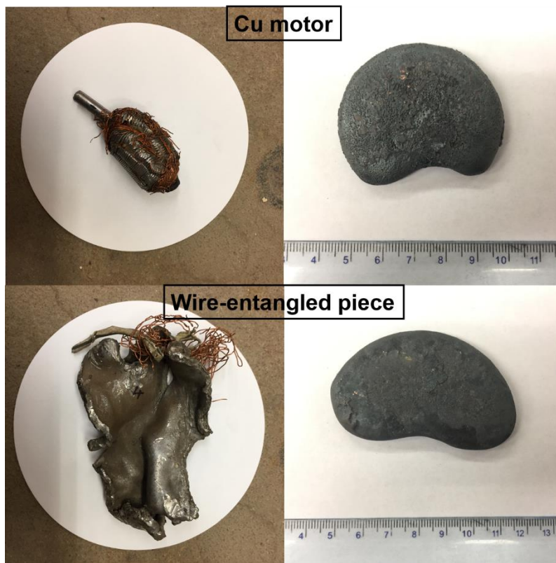
Figure 17. Collected molten melt for identified Cu source of Sample 1
