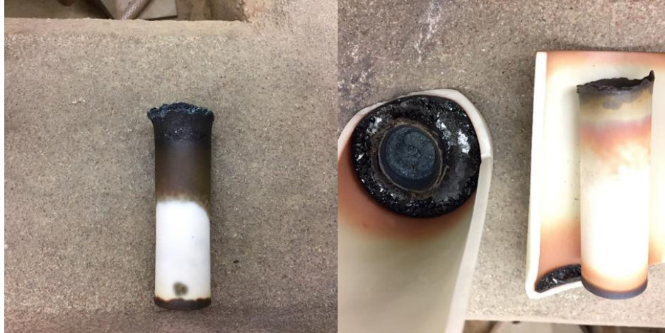
Figure 27. Broken alumina crucible after slagging experiment
