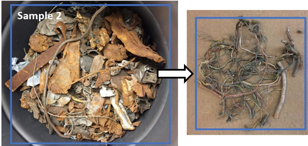
Figure 3. Steel scrap of Sample 2 and identified Cu source
